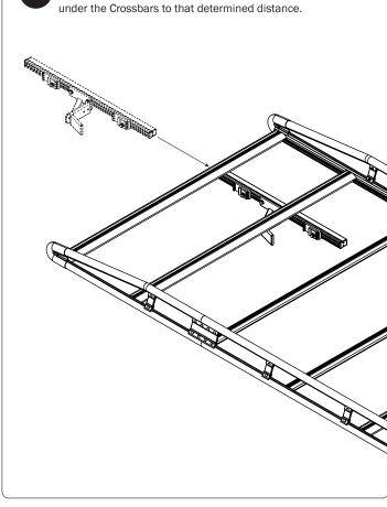
After determining Front to Rear Ladder Hook spacing
