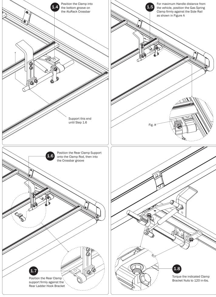
Torque the indicated Clamp Bracket Nuts to 120 in-lbs.
