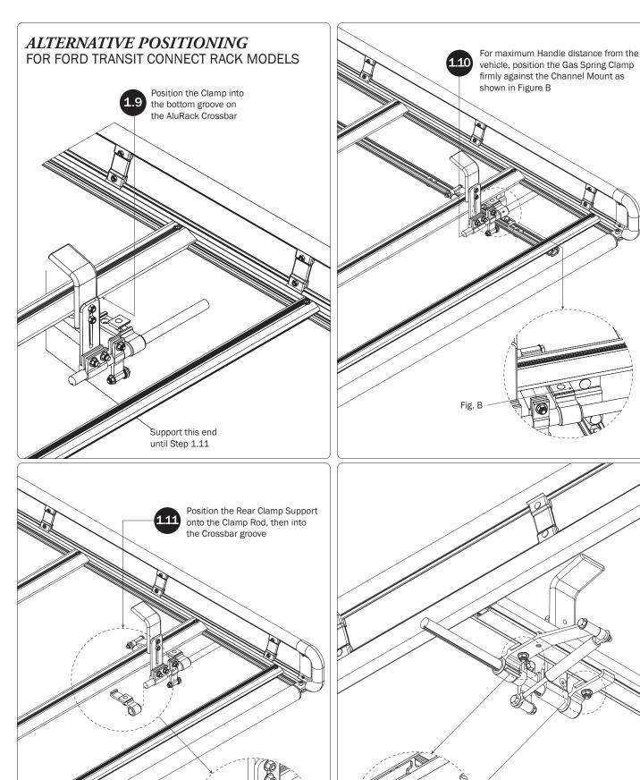
Position the Rear Clamp \ support firmly against the Rear Ladder Hook Bracket
