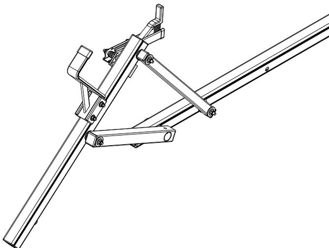
**1.4** Remove and save front Rotation and Hardware as shown.
