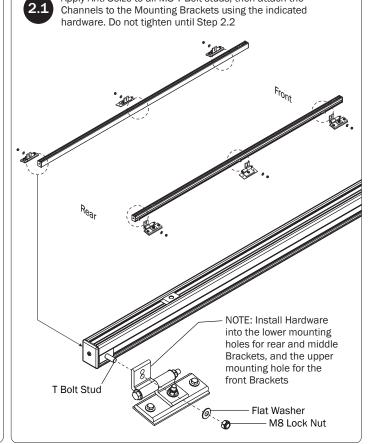
Apply Anti-Seize to all M8 T Bolt studs, then attach the
