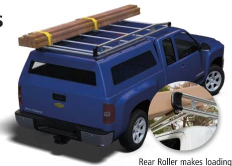
Rear Roller makes loading and unloading easy
