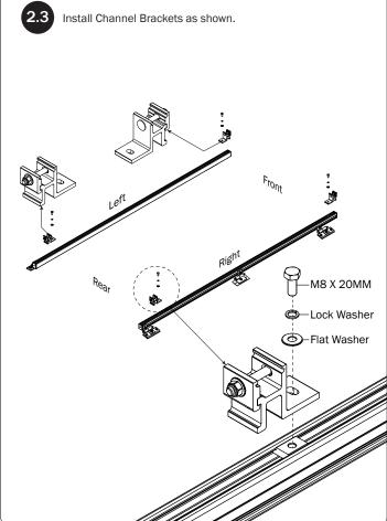
Set to distances shown below. Do not torque the Crossbar Mounting Brackets until Step 3.3–3.4. Finger-tighten them into designated dimension to hold them in place, then proceed to your Feature (FEA) Assembly Manual.
