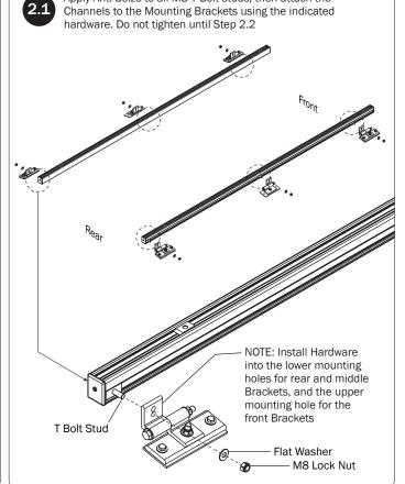
Apply Anti-Seize to all M8 T Bolt studs, then attach the
