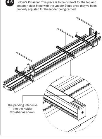
Install the Ladder Holder Padding into the top groove of the
