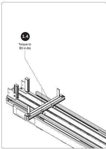
Remove the End Caps from one side of the Rear and Center Ladder Holders. Move the End Stop on that side from the Rear to Center Ladder Holder and replace End Caps as shown below.
