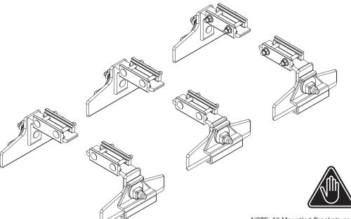
NOTE: All Mounting Brackets come pre-assembled with bolts facing the same orientation. For safety, it's recommended to position all protruding Top Clamp bolts inward. This will necessitate a partial reassemble of two of the four Mounting Brackets as shown in Steps 1.1–1.6 on pages 3 & 4.
