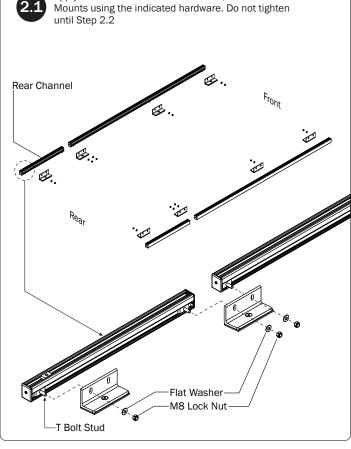
Apply Anti-Seize to all M8 T Bolt studs, then attach to
