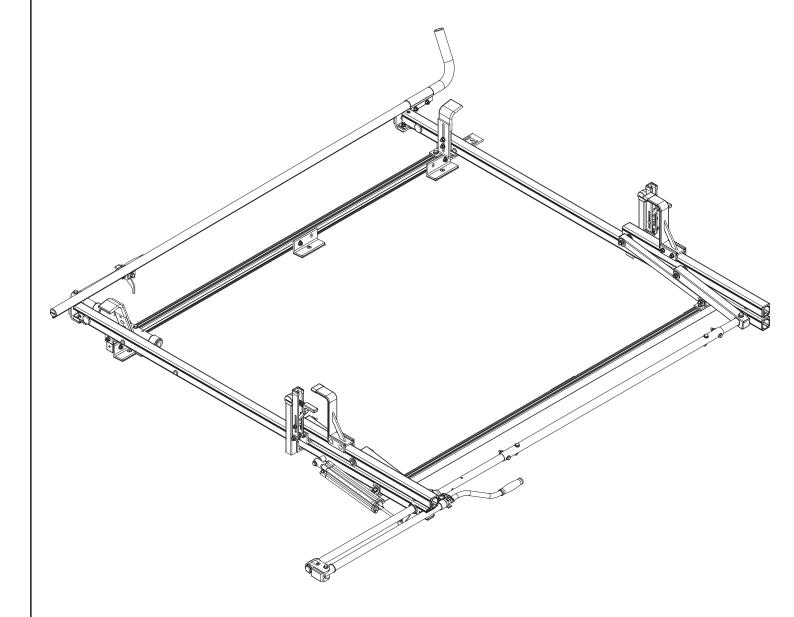
\* Note: Crossbars are not centered on the vehicle. Set Crossbars according to the LH dimensions as shown in the Assembly Manual.
