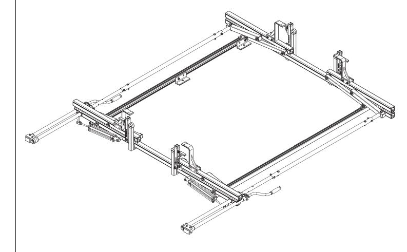
Note: Crossbars are not centered on the vehicle. Set Crossbars according to the LH dimensions as shown in the Assembly Manual.
