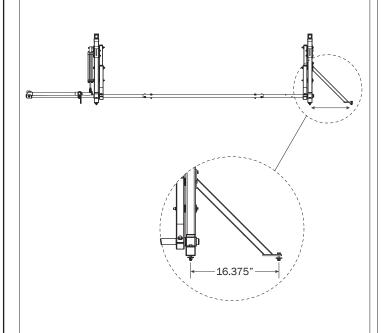
6.00 Ft: Drill holes into the Service Body mounting location according to dimensions shown.
