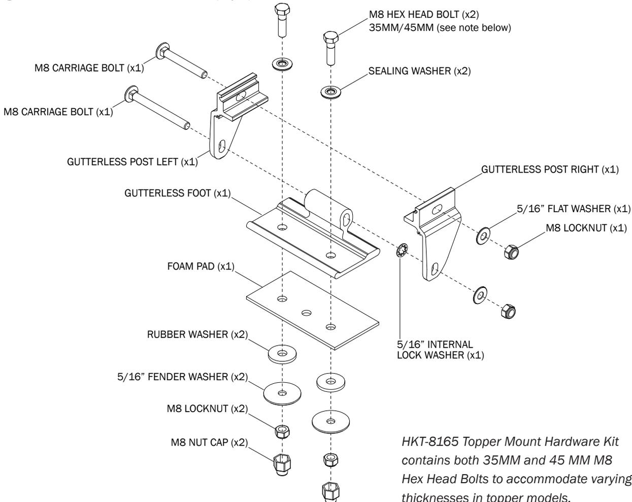
*HKT-8165 Topper Mount Hardware Kit contains both 35MM and 45 MM M8 Hex Head Bolts to accommodate varying thicknesses in topper models.*
