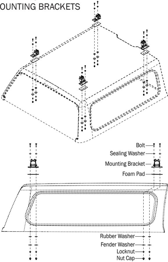
**1** Set mountings into pre-drilled holes as shown.
