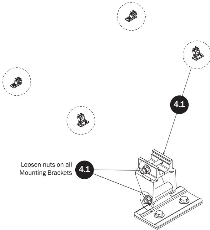
NOTE: Rack should be adjusted to attach the Mounts to Heavy Duty Crossbars only.
