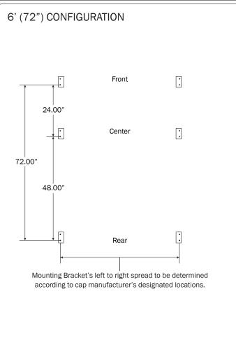
Mounting Bracket's left to right spread to be determined according to cap manufacturer's designated locations.
